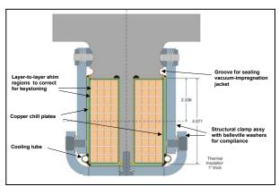
Figure 3 - Modular coil details
