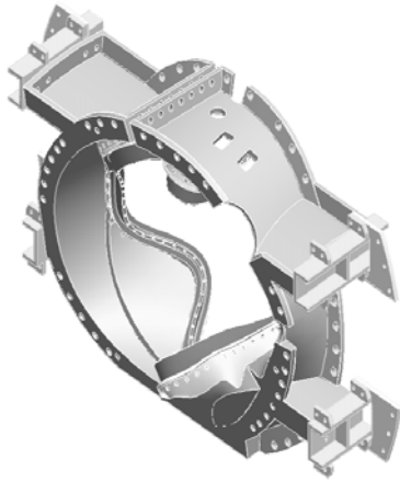
Figure 2-Mounting support brackets to casting
