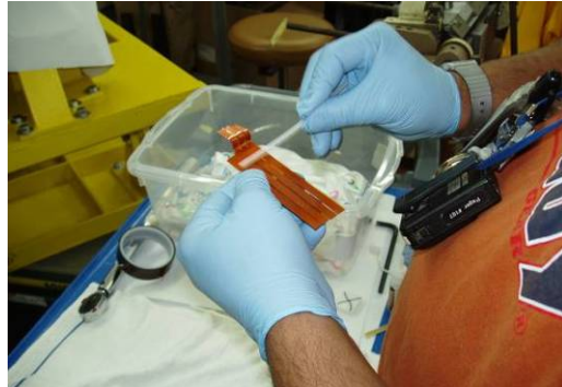
Figure 26-Applying Adhesive to Vertical Cladding
