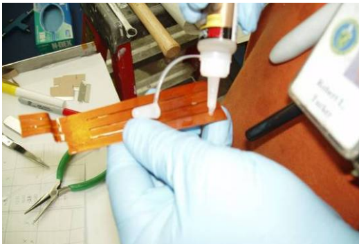
Figure 26-Applying Adhesive to Vertical Cladding
