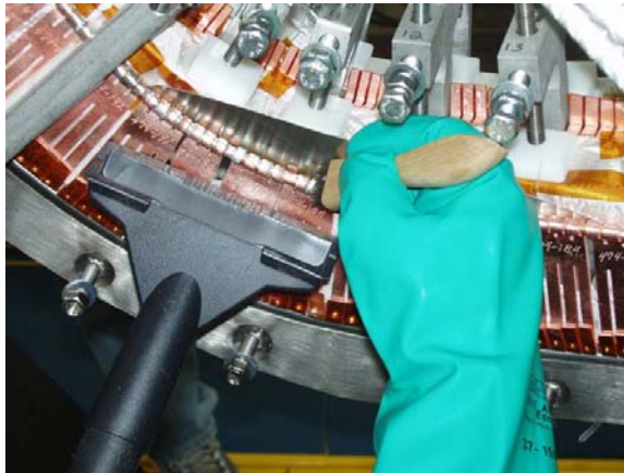
Figure 26- Cleaning of Soldered Chill Plates
