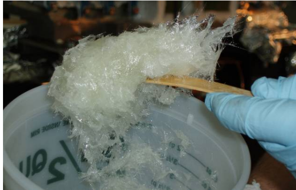
Figure 42-Epoxy/Glass Mixture- "Cotton Candy"
