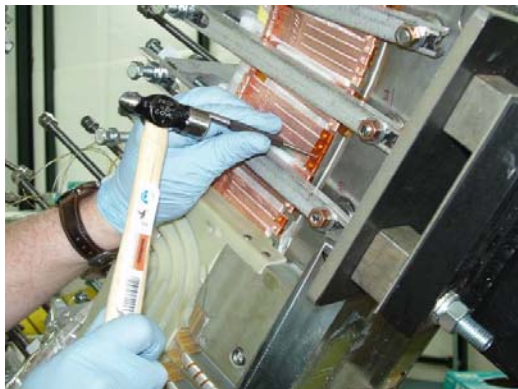
Figure 22- Staking Chill Plates
