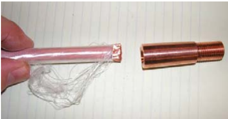
Figure 12- Removing Nylon Serve from conductor
