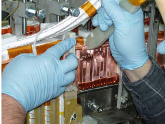
Figure 23- Setting Chill Plate and Tubing
