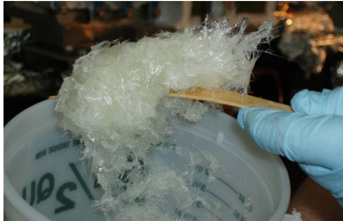
Figure 54-Epoxy/Glass Mixture- "Cotton Candy"
