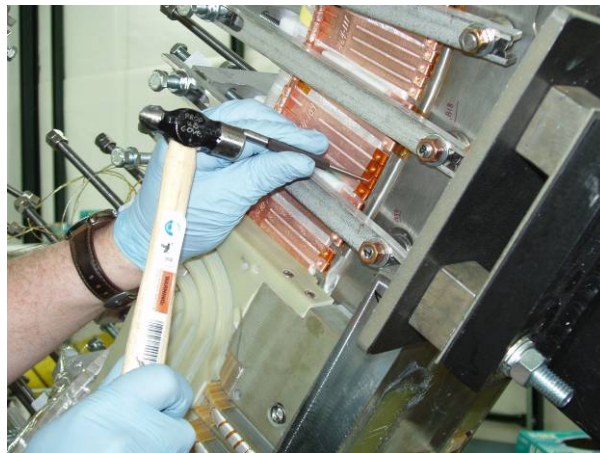
Figure 27- Staking Chill Plates
