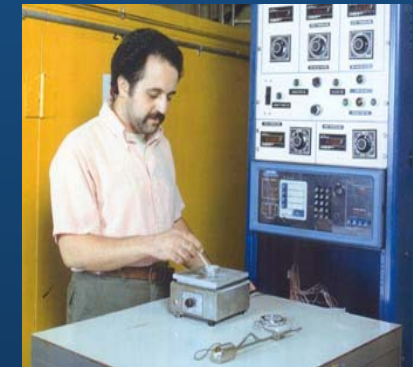
"Scrambled Egg" test to verify Gel temperature
