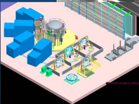
Modular coil winding & Field Period assy. area
