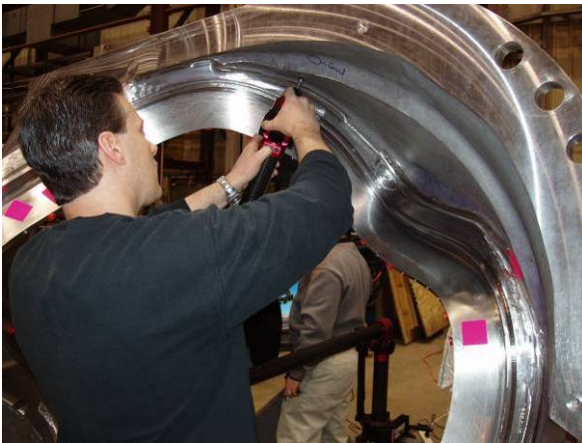
Using “Romer” Mechanical Measurement arm to verify surfaces
