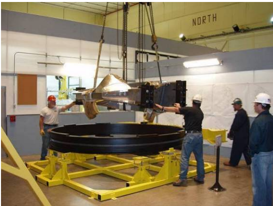
Loading Winding Form Into Support Ring
