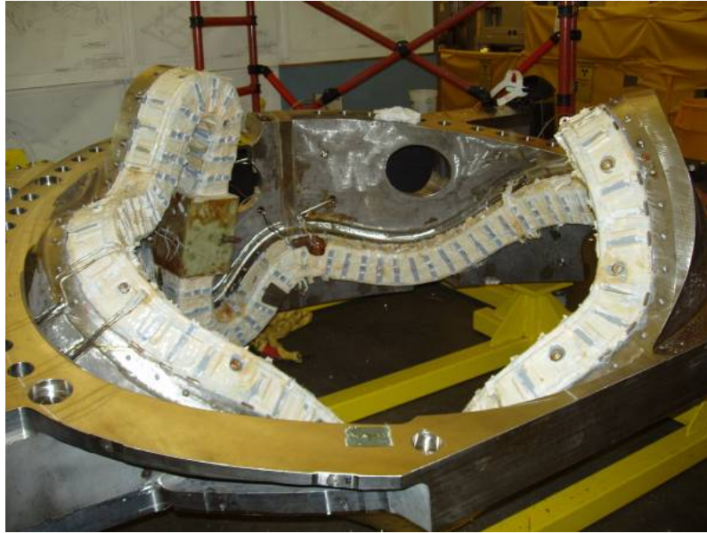
Modular Coil without the Epoxy Shell
