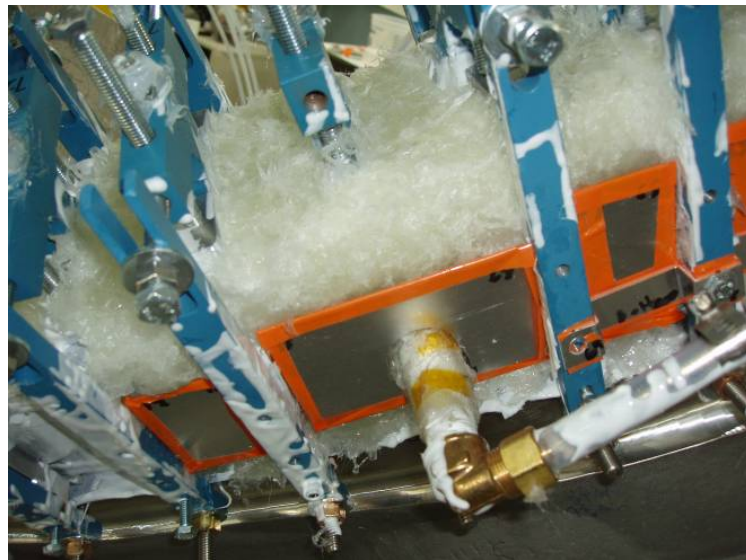
Epoxy/Chopped Glass Structural Shell
