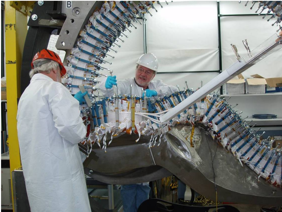
Modular Coil Winding Operation
