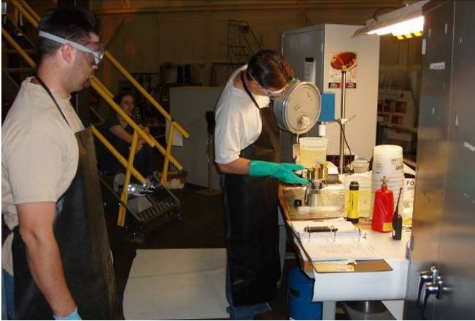
Epoxy Being Weighed prior to VPI
