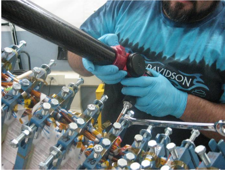
Technician measuring the location of the coil turns
