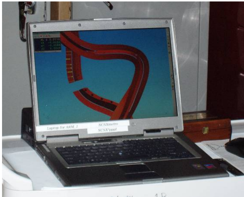
Model of coil showing measurements taken with the Romer arm
