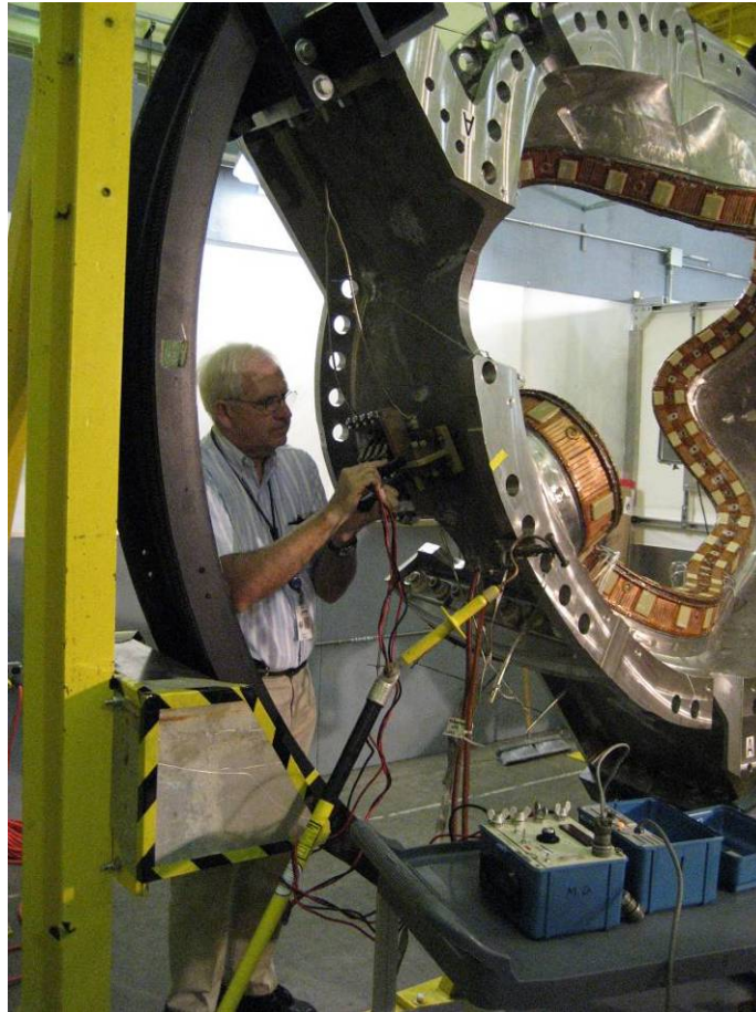
Measuring the Coil Resistance
