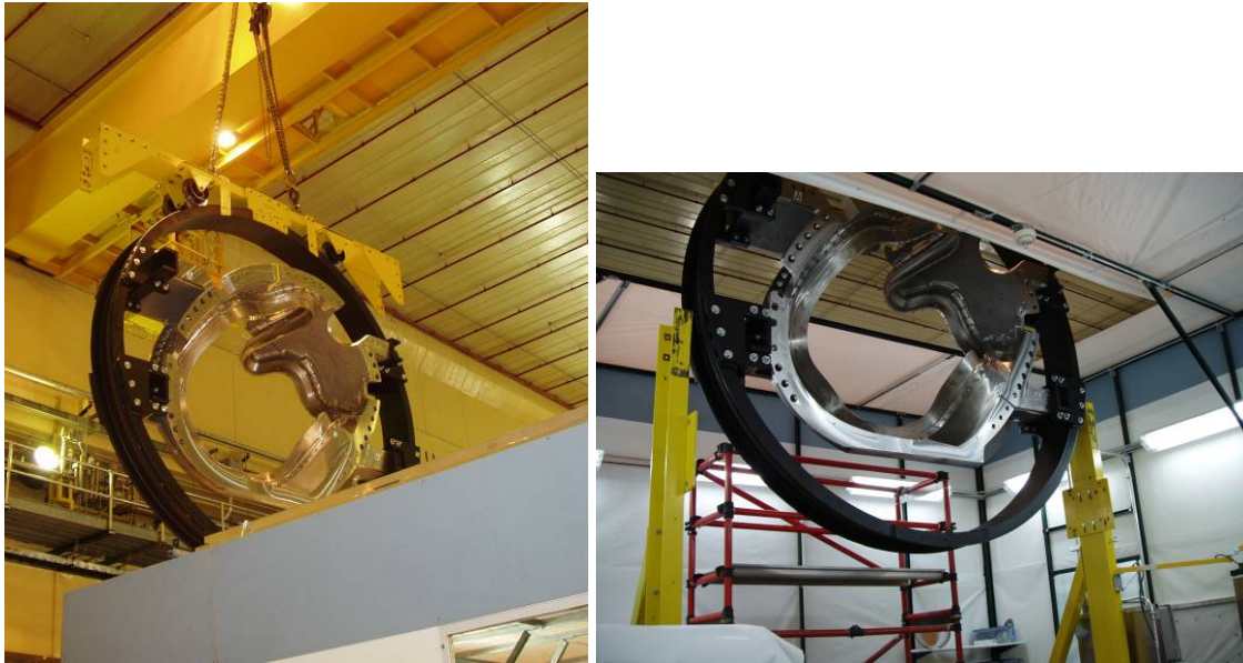
Transferring Coil Assembly to Winding Station
