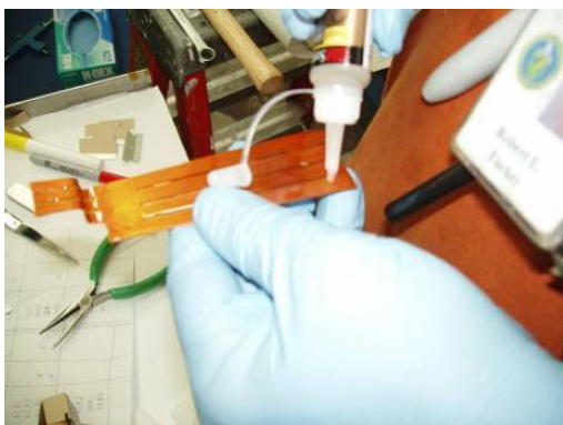
Application of 3M Adhesive to Kapton
