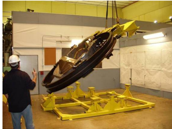
Transferring Coil to Vertical Position for Transport
