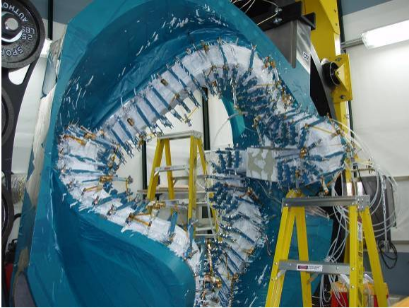
RTV over paint of the bag mold while under vacuum
