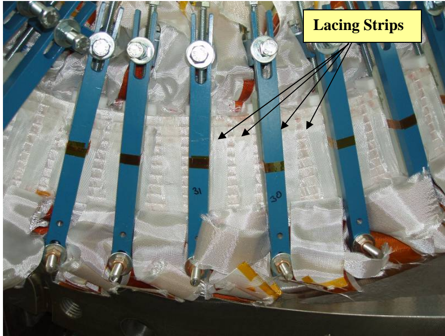
Glass Tape Lacing Strips Secured
