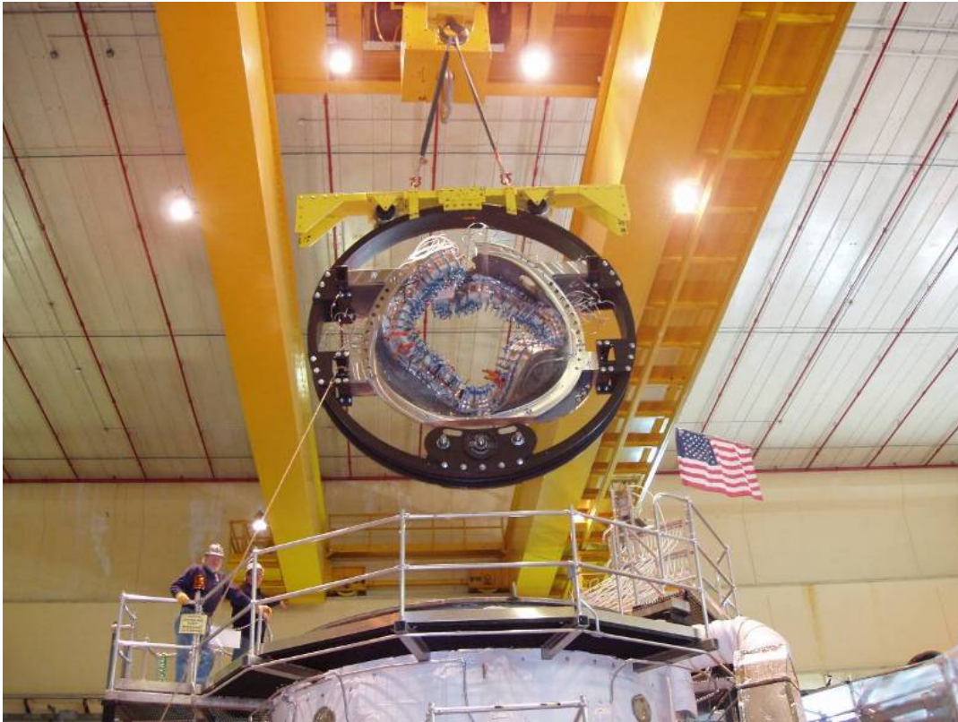
Modular Coil being lifted into the Autoclave
