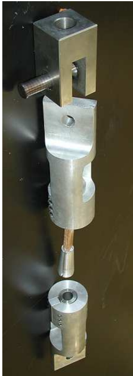
Figure 13. Assembled ISMC tension test grips and test fixturing.
