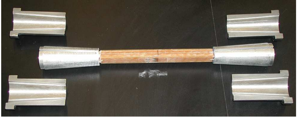
Figure 10. ISMC tension test specimen with split angular tension grips in place.
