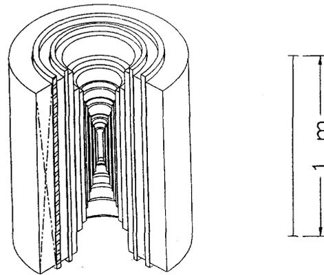
Fig. 1. Isometric drawing of the 60 tesla magnet showing the coils and the shells
