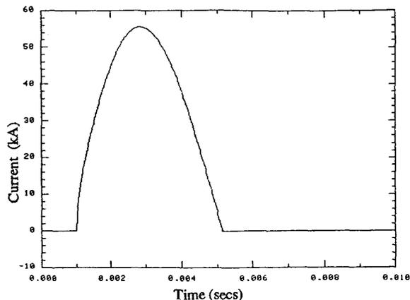
Fig. 5. Current waveform produced by the capacitor bank discharge into the coil 1 and coil 2 prototypes
