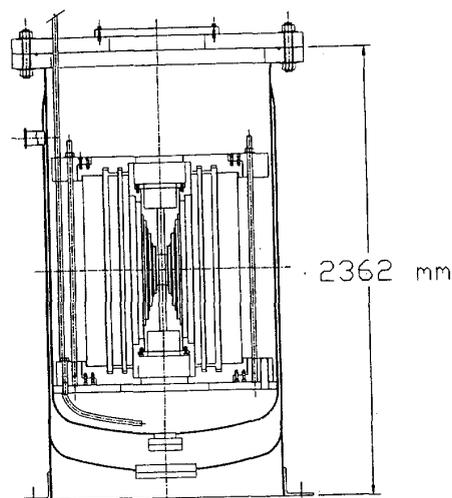
Fig. 4. Cross sectional drawing of magnet showing coil frame and dewar.
