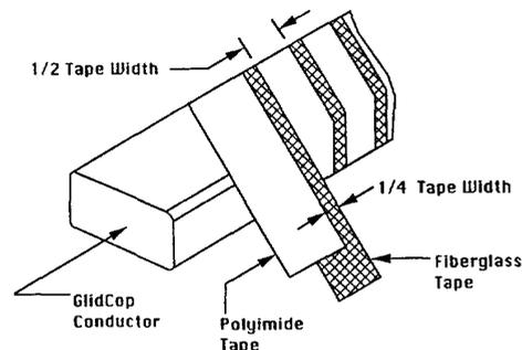
Fig. 2. Insulation wrapping about conductor. Insulation is applied as the magnet is wound.
