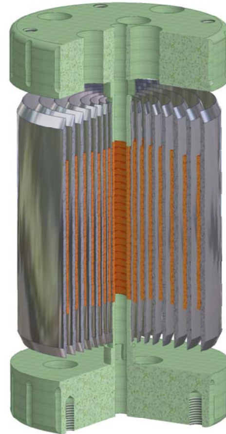
Insert reinforcement structure with zylon removed to illustrate metal placement
