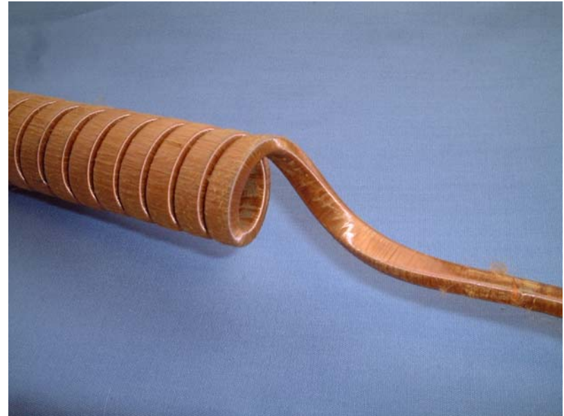
Example of zylon serving present on Cu-Nb conductor helix.
