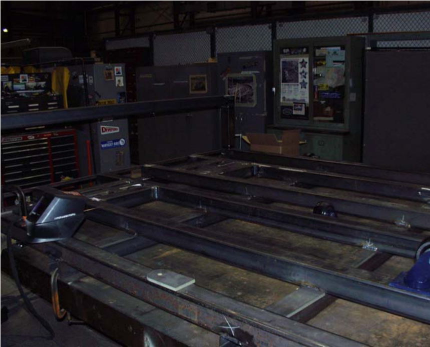
Figure 5-24 Cryostat carriage in fabrication
