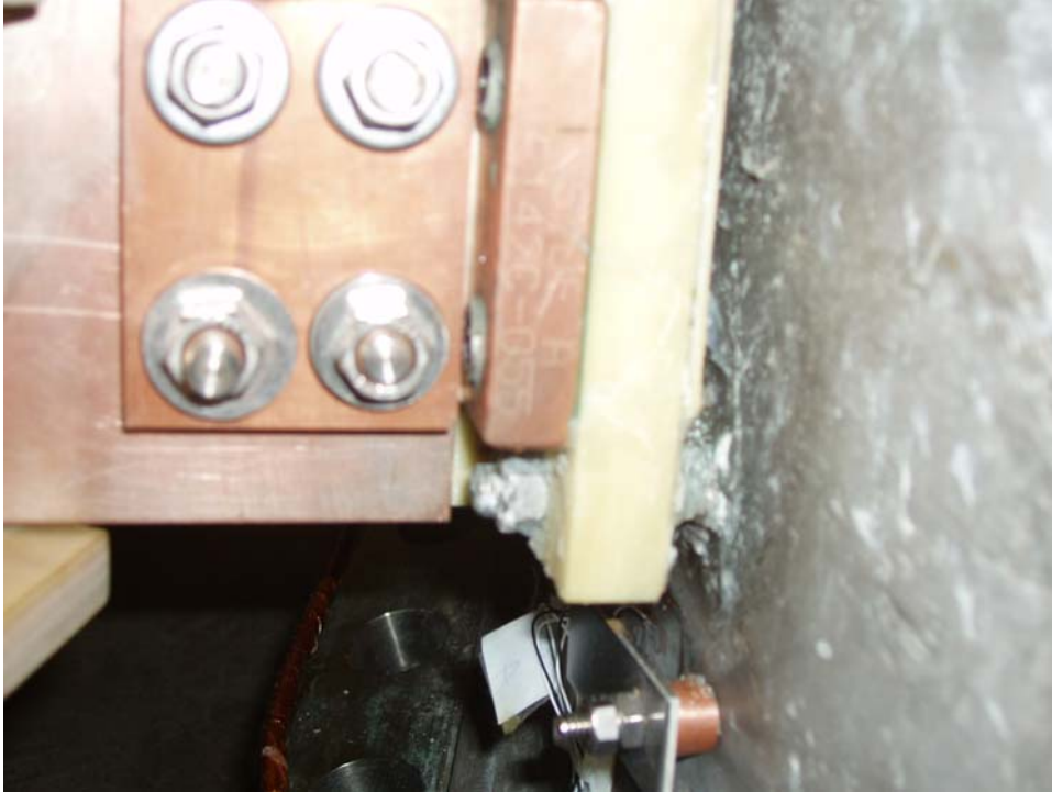
Figure 5-38 Strain gage (SG15) near lead block
