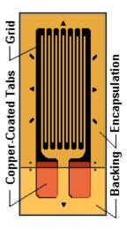
CEA-Series strain gages are polyimide-encapsulated A-alloy gages, featuring large, rugged, coppercoated tabs for ease in soldering leadwires directly to the gage. These thin, flexible gages can be contoured to almost any radius. In overall handling characteristics, for example, convenience, resistance to damage in handling, etc., CEA-Series gages are outstanding.
