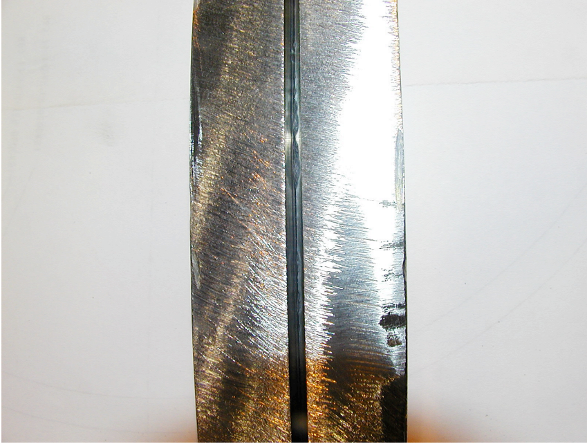
Figure 8: Backside of the joint after welding
