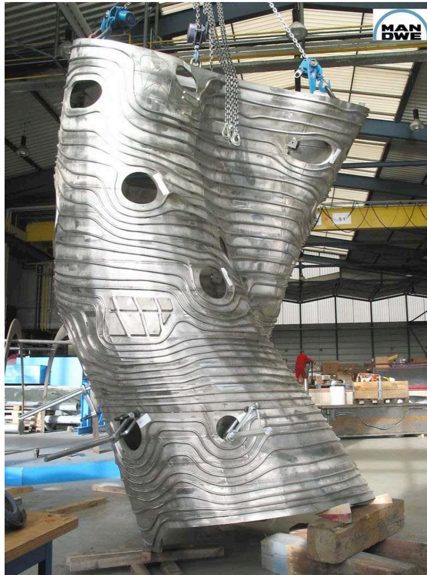
Plasma vessel with cooling pipes (MAN DWE)
