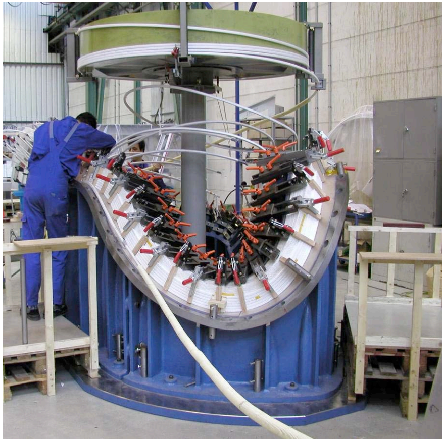
Winding of a coil (ABB, Augsburg)
