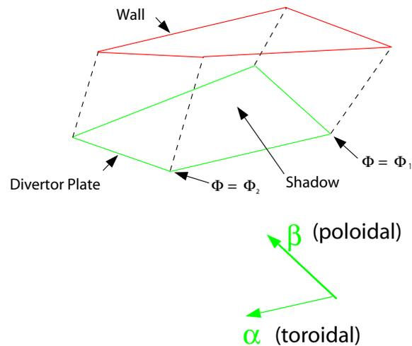
The intersection of a divertor plate with a poloidal plane is assumed to be a straight-line segment whose end-points vary linearly with toroidal angle,  $\Phi$ , sweeping out a non-planar quadrilateral surface in 3D for  $\Phi_1 < \Phi < \Phi_2$ .
