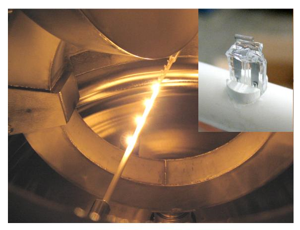
2 ceramic rods with arrays of filaments
