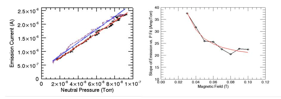
Confinement is determined by loss due to all sources (rods, classical, neo-classical...). The rods are a major source but other sources are significant:
