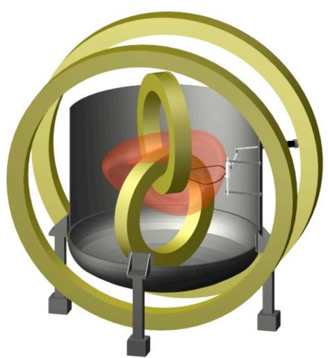
Magnetic surfaces are created from only four circular coils<sup>1,2</sup>
