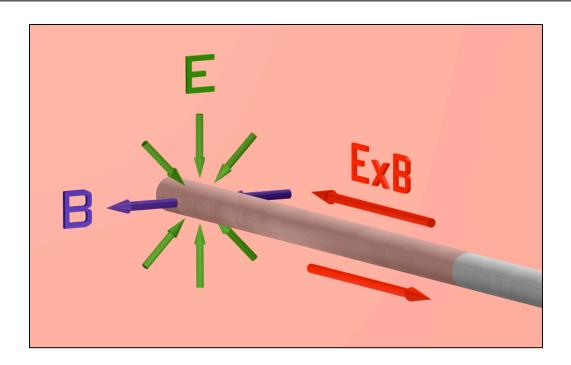
Insulated rods charge up negative relative to plasma Resulting ExB drift pattern convects particles along the rod all the way to the open field lines
