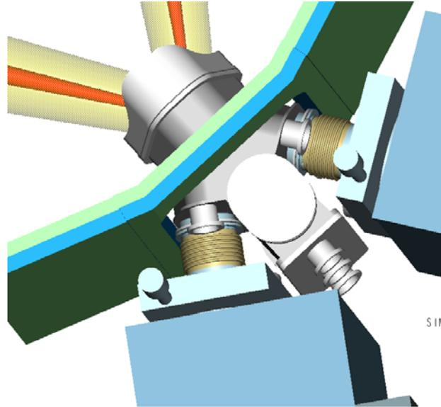
**Figure 4-1 Neutral beamlines connected to Auxiliary Systems duct**
