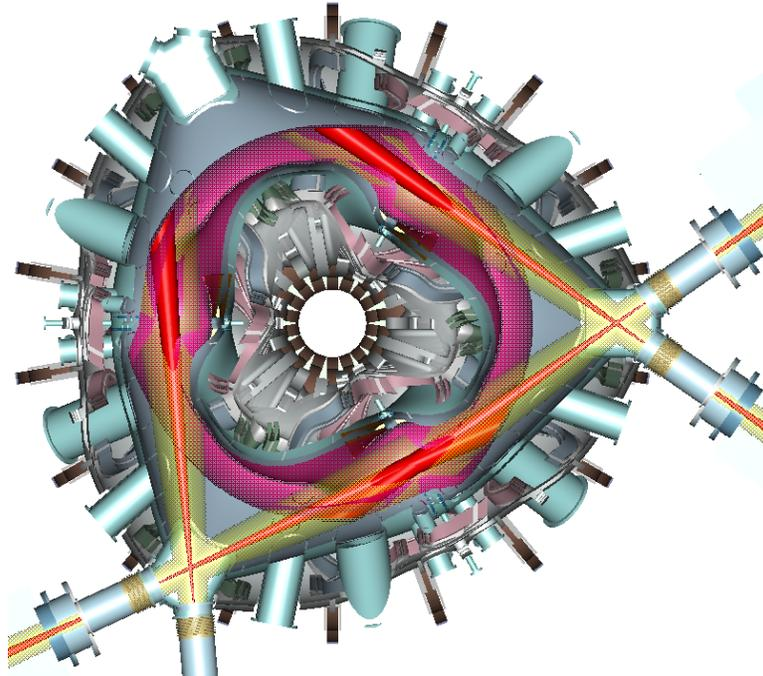
**Figure 4-2 Plan view of beam injection into plasma**
