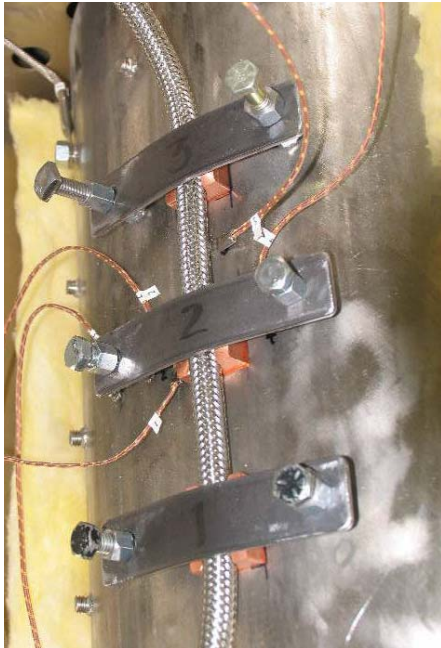
Test article, 3 saddle clamps on curved surface
