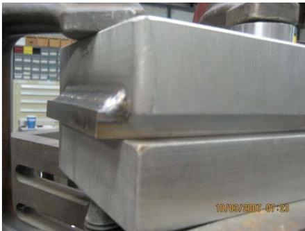
*This welding concept minimizes weld shrinkage forces between the flanges and provides a load path as near as possible to the shell-to-shell interface.*
