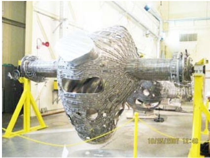
Station 1 – Vacuum Vessel (VV) Prep
