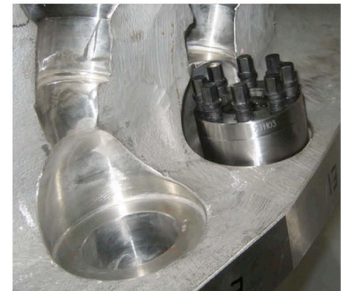
Studs tensioned to 74 kips using tensioning nuts from Superbolt
