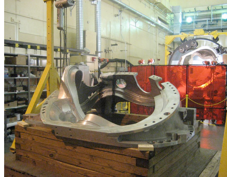
Modular Coil Winding Forms ($9M) completed June, 2007
