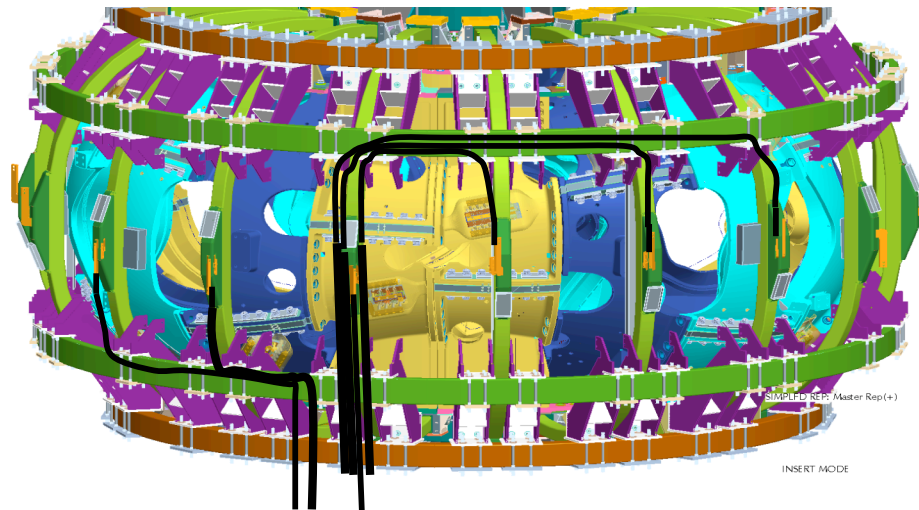
MC Lead stub connections shown on Station 6
