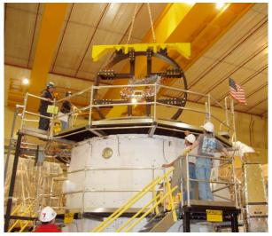
FY06 Modular Coil Manufacturing Plans-Complete Winding (7) and VPI (6)
