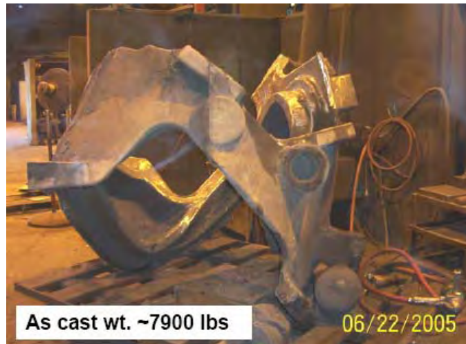
Fig. 7. QPS Prototype Modular Coil
