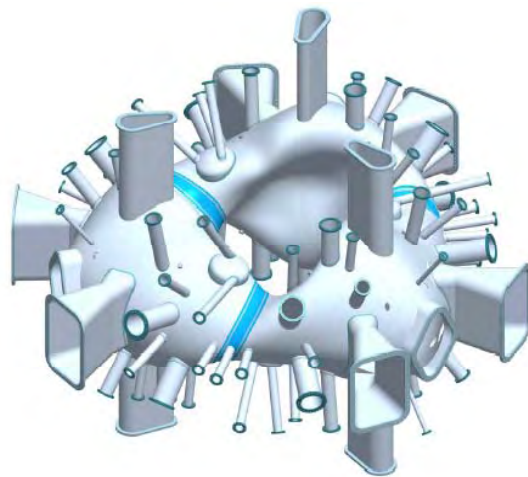
Fig. 2. NCSX vacuum vessel design.
