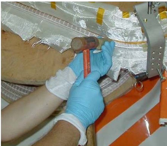
Figure 3- Setting Turns in Position
