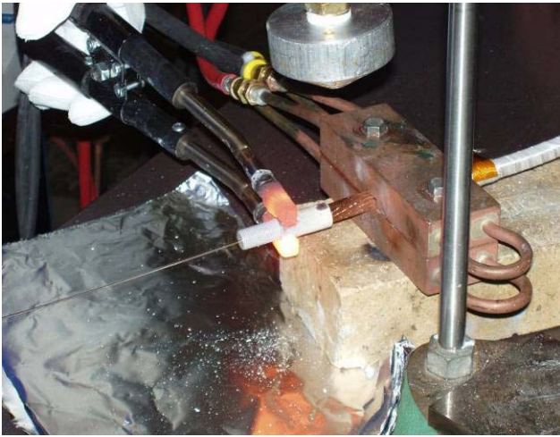
Figure 10- Brazing of Conductor Leads
