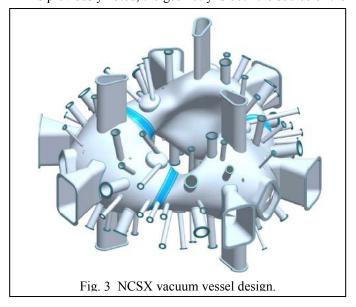
compact stellarator's physics benefits as well its key engineering challenge. The aim of the NCSX construction project is the accurate realization of the unusual geometries required of the magnets, vacuum vessel, and associated structures. The adopted project strategy has two parts: 1) development of critical manufacturing processes through R&D prior to production, and 2) management of requirements flow-down from physics specification to finished product through system engineering.
