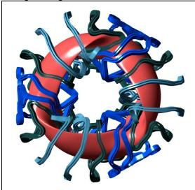
Fig. 1 NCSX plasma and modular coils.
