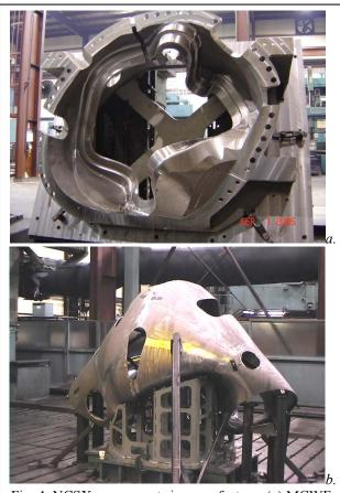
Fig. 4. NCSX components in manufacture: (a) MCWF, (b) vacuum vessel.
