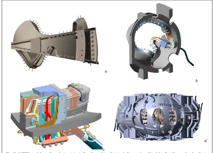
Fig. 2. NCSX modular coil set design. (a) winding form, (b) coil, (c) winding pack and lead details, (d) completed coil set..
