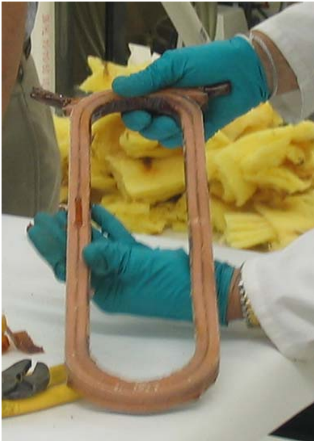
Figure 8 Practice coil vacuum impregnated with cyanate ester
