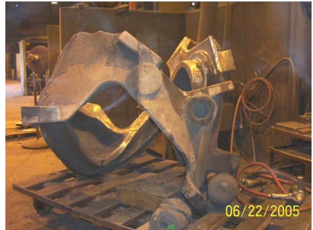
Figure 6 Prototype casting prior to machining
