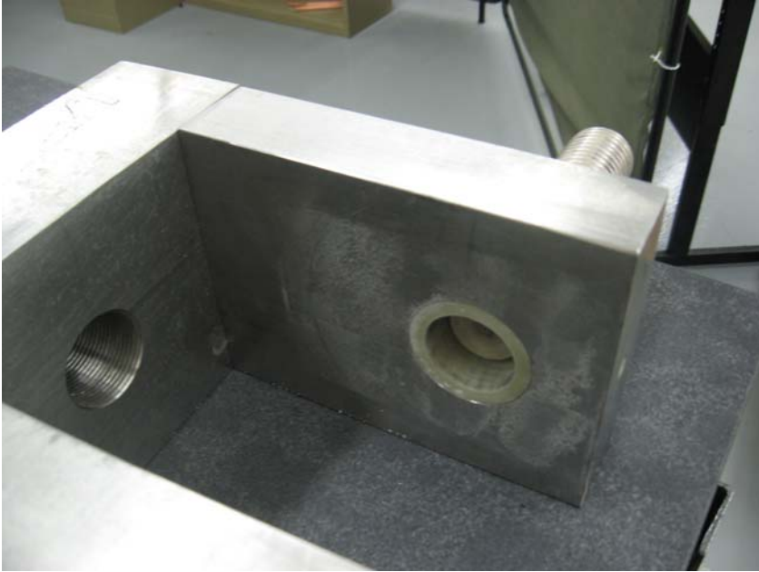
Outer trunnion showing powder after completion of testing.
