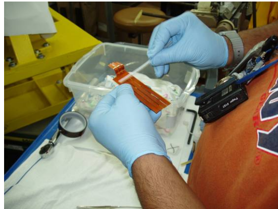
Figure 25-Applying Adhesive to Vertical Cladding
