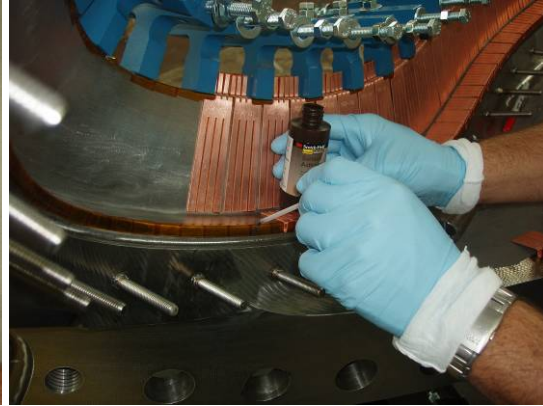
Figure 29- Applying Accelerator [Horizontal]
