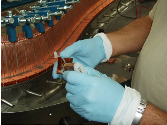
Figure 28- Applying Adhesive to Horizontal Cladding
