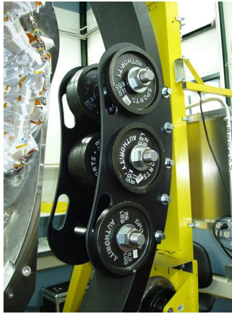
Figure 8-Modular Coil Counter Balance Assembly
