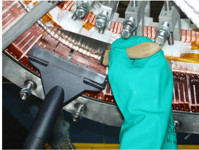
Figure 32- Cleaning of Soldered Chill Plates
