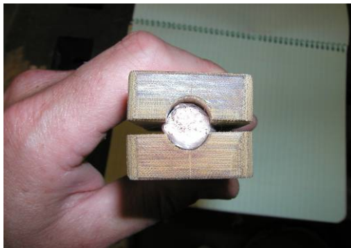
Figure 13-Conductor in Forming Block
