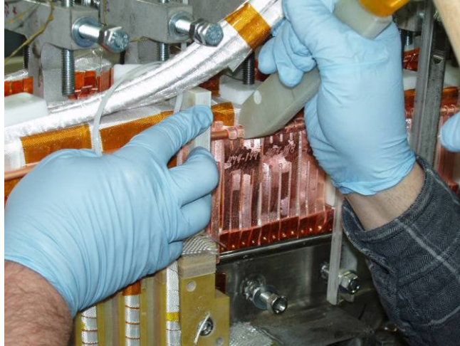
Figure 29- Setting Chill Plate and Tubing
