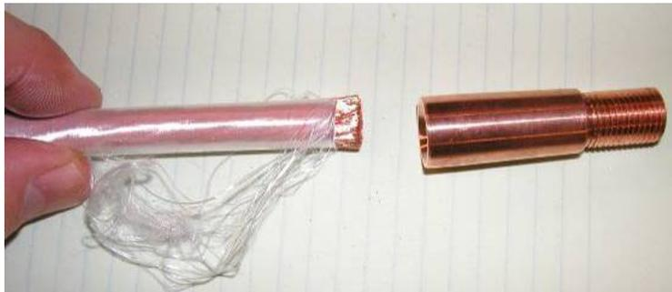
**Figure 14- Removing Nylon Serve from Conductor**
