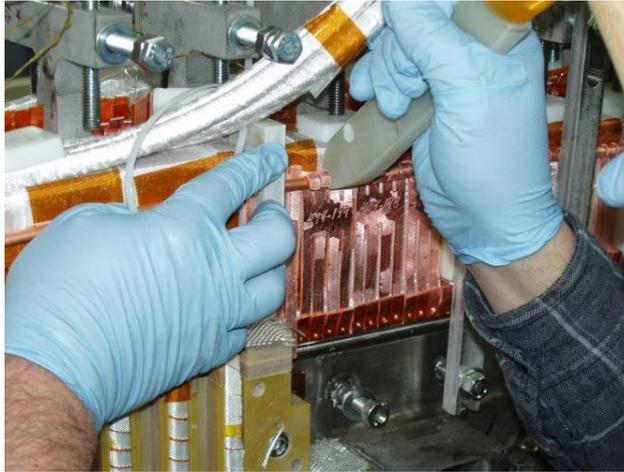
**Figure 29- Setting Chill Plate and Tubing**
