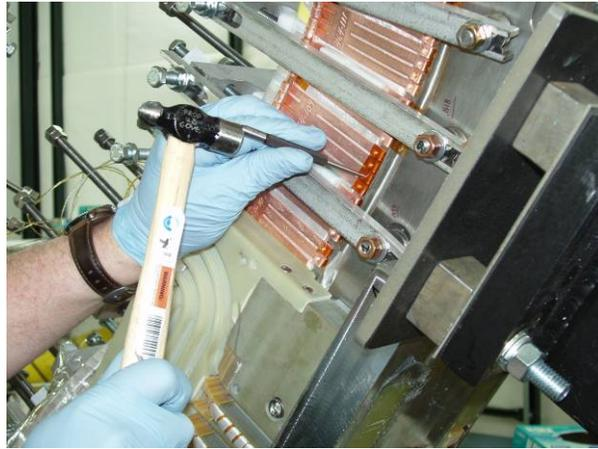
**Figure 27- Staking Chill Plates**
