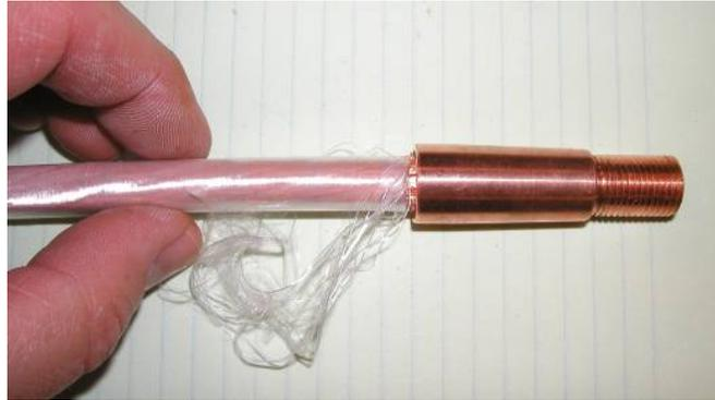
Figure 15- Conductor in Connector
